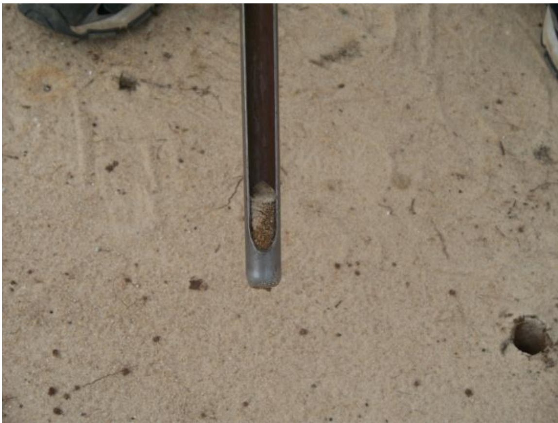
Figure 4-4. Soil corer (2 cm diameter) used to take soil samples at a depth of 5 cm.
